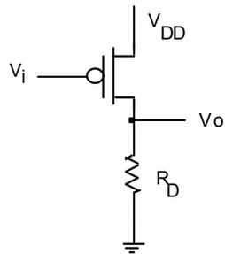
Para  $V_i = 0 \text{ V} = "0"$   $V_o = V_{DD} = "1"$
