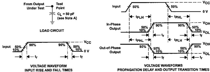
NOTES: A. C<sub>L</sub> includes probe and test-fixture capacitance.
