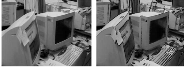
Fig. 2. Edge enhancement. Image on the left is the original video frame; image on the right is the processed frame by edge enhancement. The example image has been captured from the actual VGA output of the FPGA board.
