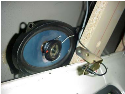
Figure 4. Detail of error microphone and secondary source.
