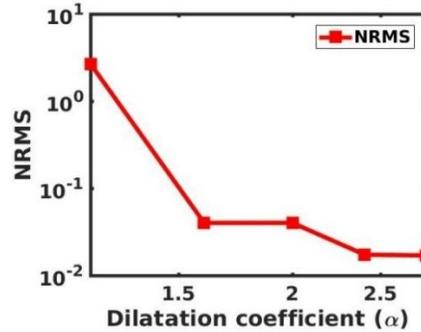
**Figure 2.** Normalized Root Mean Square (NRMS) error convergence for varying dilatation coefficient  $\alpha = \{1.2 \ 1.6 \ 2.0 \ 2.4 \ 2.8\}$  and nodal spacing  $h = 0.04$  cm
