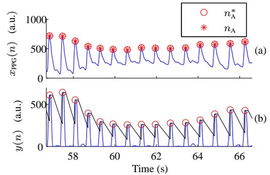
Figure 1. Example of detector behaviour during a DAP event: (a) shows the PPG signal, and (b) shows its SSF (blue) and the resulting time varying threshold (black).
