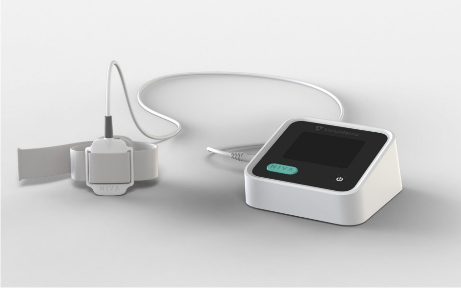
Figure 5: NIVA device. This device designed by Volumetrix (Nashville, TN) measure the changes in PVP in the wrist using a piezoelectric sensor. From [26].
