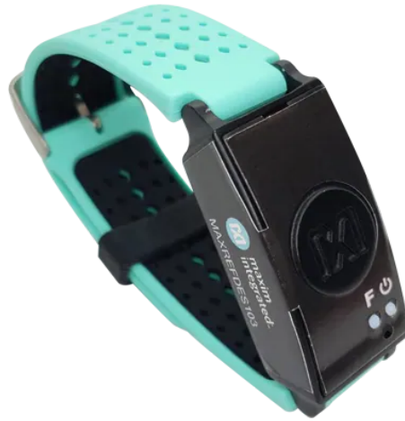
Figure 50: Maxim MAXREFDES103 [1]. A wrist-worn device capable of recording PPG with red, green, and infrared channels.
