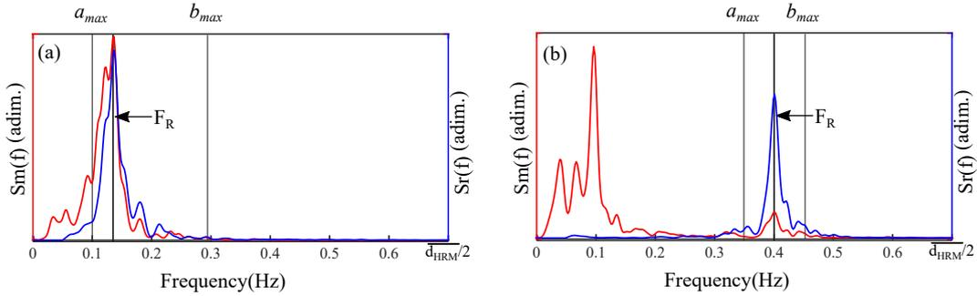
Figure 3.6: Correlation between  $S_m(f)$  and  $S_r(f)$  in two particular cases: (a)  $F_R$  is below 0.15 Hz and (b)  $F_R$  is 0.40 Hz.
