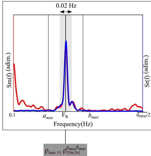
Figure 3.1: Diagram of the SCHF methodology: PSD of  $m(t)$  ( $S_m(f)$ ) and PSD of  $r(t)$  ( $S_r(f)$ ). The correlation between  $S_m(f)$  and  $S_r(f)$  was calculated by expanding symmetrically the  $[a, b]$  range in steps of 0.02 Hz per iteration. The maximum value of the correlation between  $S_m(f)$  and  $S_r(f)$  ( $\rho_{max}$ ) determines the lower and upper limits  $[a_{max}, b_{max}]$  of the redefined HF band ( $HF_{SC}$ ).
