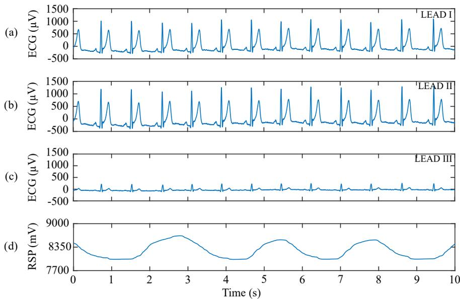
Figure 2.1: Ten seconds of the simultaneous recorded signals: (a) ECG Lead I, (b) ECG Lead II, (c) ECG Lead III, and (d) RSP.
