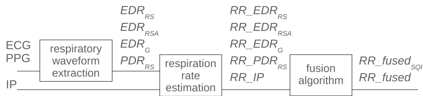
Figure 2. Computation of RR series: first, surrogate respiratory signals were derived from ECG and PPG waveforms; then, RRs were estimated from respiratory signals using an AR model; finally, robust RR estimates were computed by combining the individual RR estimates with a fusion algorithm.
