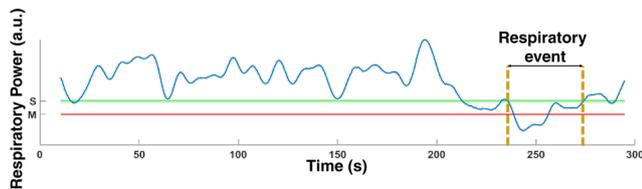
Fig. 1. Example of a 5-min segment where a respiratory event is detected. The blue line represents the estimated respiratory power from combinatorial analysis of EDR signals, and the event is detected based on the green line (selection level, S) and red line (minimum level, M).
