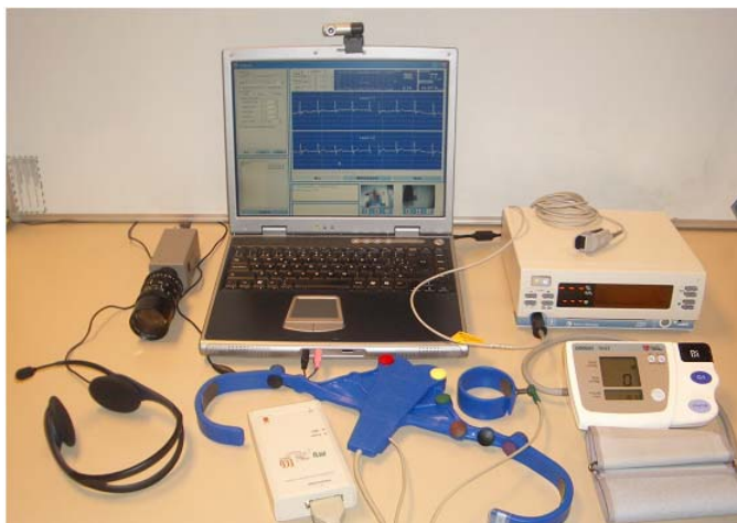
Fig. 1. Telemonitoring application designed for a mobile ICU using an UMTS access, which includes specific real-time transmission modules.
