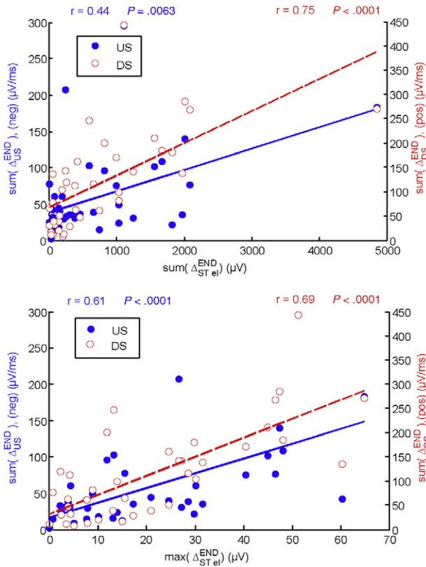
Fig. 6. Correlation between QRS slope changes (US and DS) and ST elevation. Dashed line represents DS. sum US (neg) indicates the sum of negative US change in all leads at the end of PCI; sum DS (pos), the sum of positive DS change in all leads at the end of PCI; sum ST el, the sum of ST elevation in all leads at the end of PCI; max ST el, maximal ST elevation in any lead at the end of PCI.
