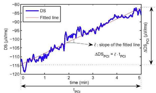
Fig. 2. Representation of the strategy by which a line is fitted to the averaged DS values during the PCI procedure in a least square sense to reduce the effect of possible outlier measurements on the DS change computation.
