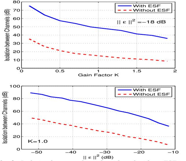
Fig. 3. Isolation between channels with and without ESF in the closed-loop subsystems.
