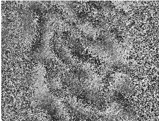
Figure 5. Phase difference map obtained from an undeformed object with the object beam travelling 20 mm in liquid nitrogen.
