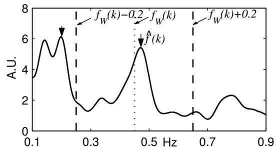
Figure 3. Interval-restricted peak search in the  $k$ -th averaged spectrum. Arrows show the selected peaks in the whole and restricted interval, respectively. Interval limits are marked with dashed lines and  $f_W(k)$  with a dotted line.
