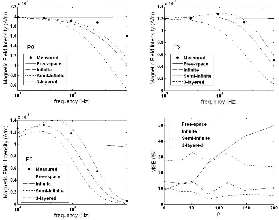
Figure 2: Computed and measured magnetic field intensity for P0, P3 and P6. The figure at the bottom right corner presents the mean squared error (MSE).
