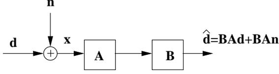
Figure 1. Linear reduced rank approximation of noisy signals.
