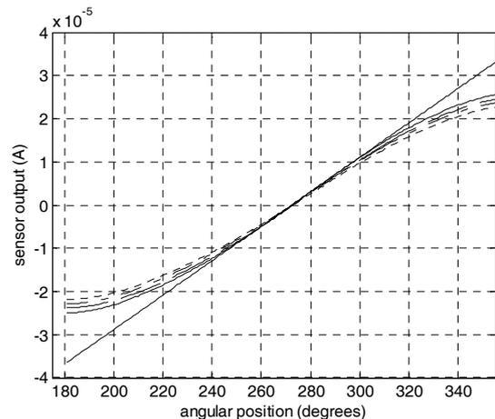
Fig. 6. GMR sensor output at 293 K (solid line), 313 K (dashed line), 333 K (dash-dot line) and 353 K (dotted line)
