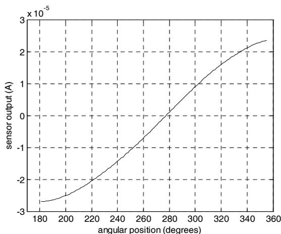
Fig. 1. Giant magneto-resistive sensor behaviour
