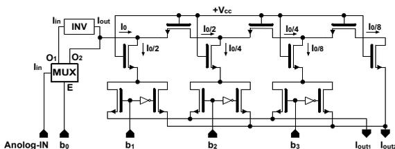
Fig. 3. Current-based analog-digital multiplier circuit
