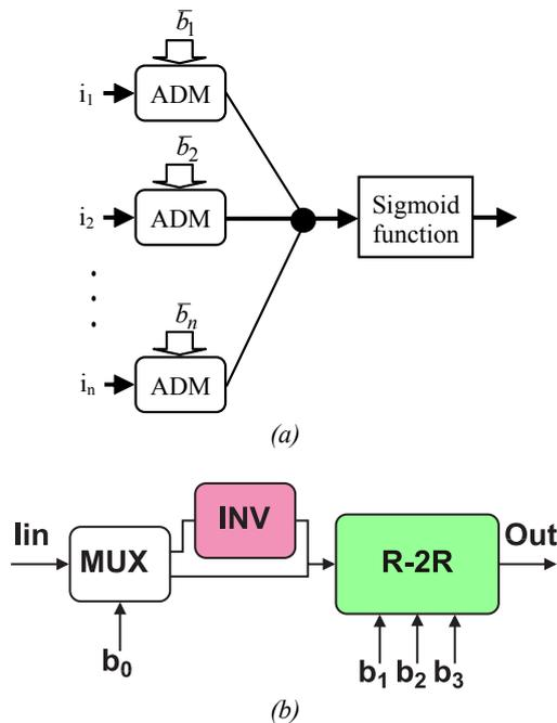
Fig. 2. Neuroprocessor architecture. (a) main building blocks; (b) analog-digital multiplier architecture
