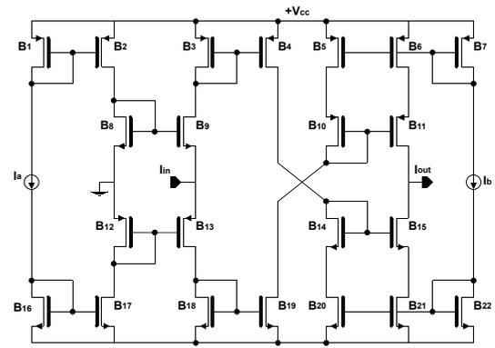
Fig. 4. Current-based hyperbolic tangent function
