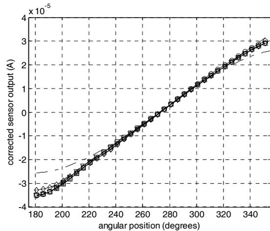
Fig. 10. Linearized sensor outputs for sensor at 293 (circles), 313 (triangles), 333 (squares), and 353 (diamonds) kelvin degrees, compared to the actual sensor output at 293 K degrees (dash-dot line)
