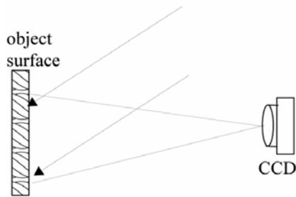
**Fig. 9:** Set-up for Speckle photography
