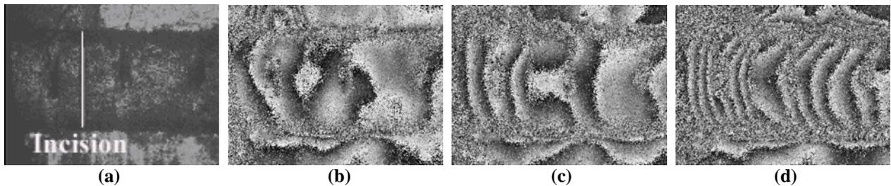
**Fig. 7.** **(a)** Aspect of sample B showing the mechanical incision. The fringe patterns have been obtained at a temperature in which  $I_C=2\text{A}$  and the applied current is 15 A after **(b)** 21 s, **(c)** 30 s and **(d)** 50 s.
