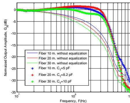
Fig. 7. Frequency response of the analog front-end.
