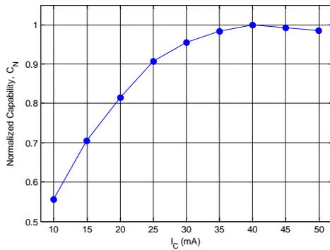
Fig. 4. Normalized TIA capability as a function of the bias current.
