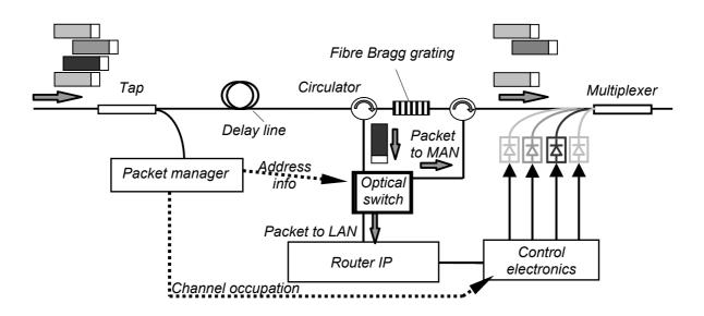
Figure 2. Access Point proposed design: every packet crossing the node suffers a delay introduced in order to avoid collisions with those packets added by the node. Additionally, packets belonging to the node's own wavelength cross the optical switch and are redirected either to the router (i.e. dropped) or again to the MAN ring.
