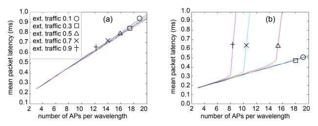
Figure 4. Mean packet latency versus number of nodes per internal wavelength for different external-tointernal traffic ratios for the internal wavelengths (a) and for the external wavelength (b).
