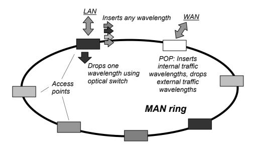
Figure 1. MAN ring proposed: each AP connects a LAN to the ring, POPs provide connectivity to and from the WAN.
