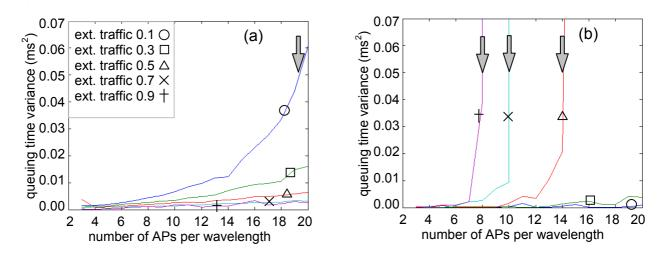
Figure 3. Queuing time variance versus number of nodes per internal wavelength, for the internal wavelengths (a) and for the external wavelength (b).
