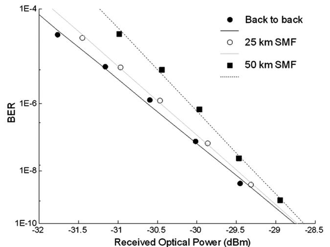
Fig. 11. BER for the downstream narrow-FSK signal (solid circles) back to back, with (open circles) 25 km, and (squares) 50 km of standard SMF obtained using the setup shown in Fig. 7.
