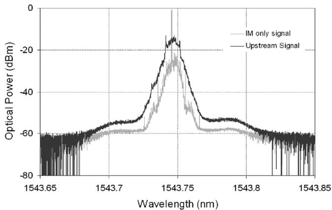
Fig. 9. Optical spectra of the upstream channel signal and of a pure-intensity-modulated signal.
