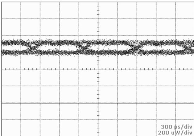
Fig. 4. Eye diagram of the downstream narrow-FSK signal before the filter.
