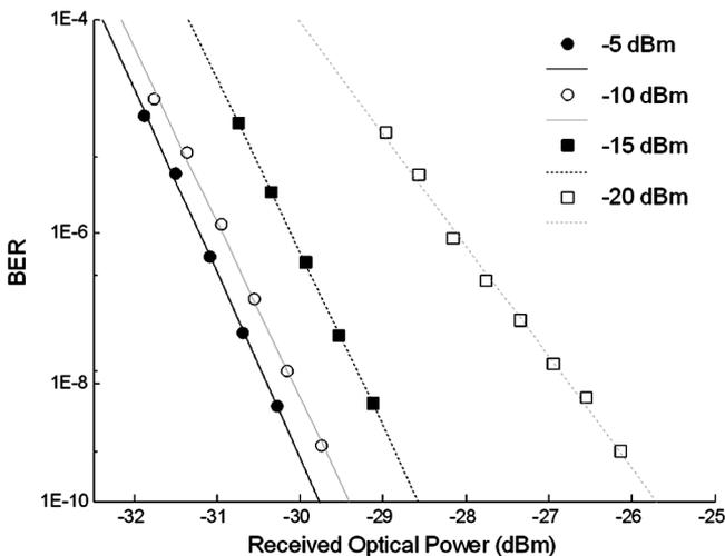
Fig. 13. Back-to-back BER for the upstream channel obtained with the setup in Fig. 7 with an optical filter in the OLT end for different RSOA input powers.
