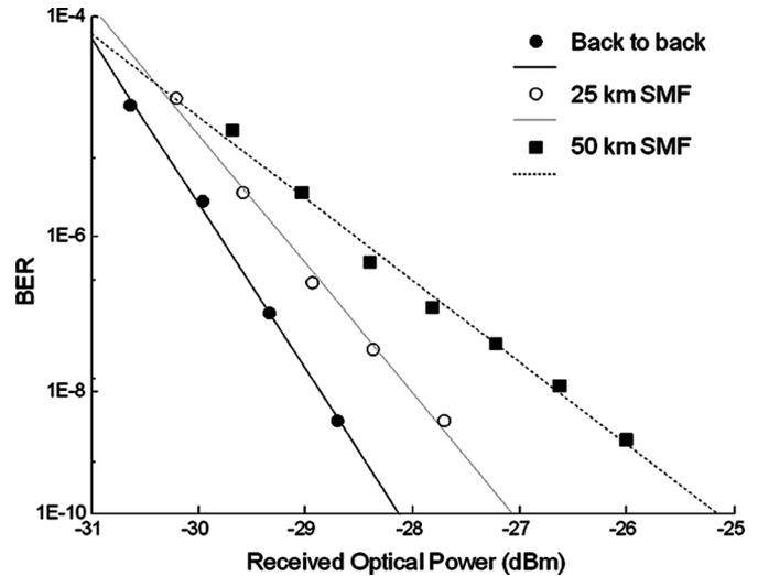
Fig. 14. BER (back-to-back, 25 km, and 50 km SMF) for the upstream channel with equal attenuations for the downstream and upstream links obtained using the setup shown in Fig. 7 including the WDM optical filtering, as in Fig. 13.
