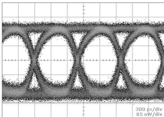
Fig. 5. Eye diagram of the downstream filtered narrow-FSK signal.
