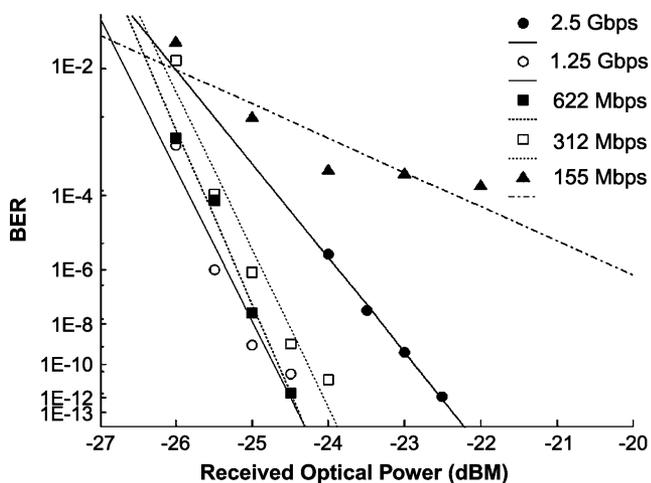
Fig. 6. Narrow-FSK BER curves as a function of received optical power measured for different bit rates using the setup shown in Fig. 2.
