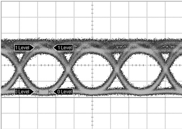
Fig. 8. Eye diagram of the upstream channel.
