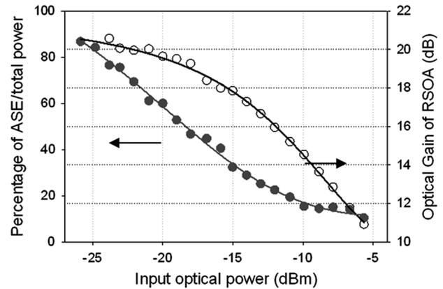
Fig. 10. (solid circles) Gain and (open circles) ASE/total power ratio of the RSOA versus input optical power.
