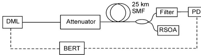
Fig. 2. Experimental setup for the measurement of narrow-FSK BER characteristics.
