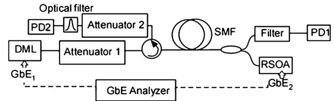
Fig. 7. Experimental setup for the characterization of the upstream channel and complete link using GbE (1.25 Gb/s) channels.
