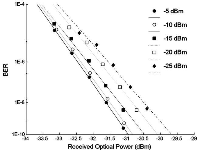
Fig. 12. Back-to-back BER for the upstream channel obtained with the setup in Fig. 7 without the optical filter in the OLT end for different RSOA input powers.
