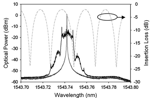
Fig. 3. Measured optical spectra of a (dark gray line) CW DFB, (black line) a narrow-FSK-modulated signal, and (dashed line) insertion loss of the demodulator.
