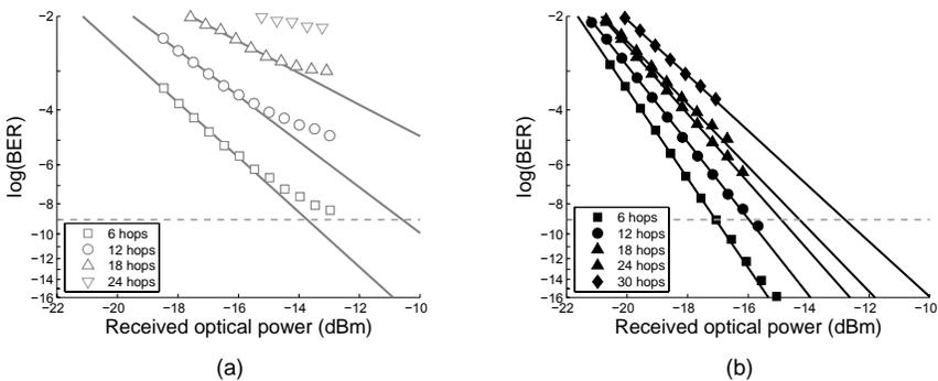
**Figure 2:** Payload BER vs. received optical power curves for two of the four considered node designs: (a) configuration A2 and (b) configuration B1.
