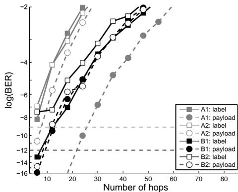
Figure 4: Scalability limits for the considered configurations. Total launched optical power = 5 dBm (-4 dBm per channel).
