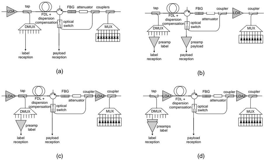
**Figure 1:** Node configurations considered. Configurations A1 (a) and A2 (b) include one in-line amplifier per node, while configurations B1 (c) and B2 (d) include two in-line amplifiers per node. One or more preamplifiers are placed before detection in order to meet the sensitivity requirements.
