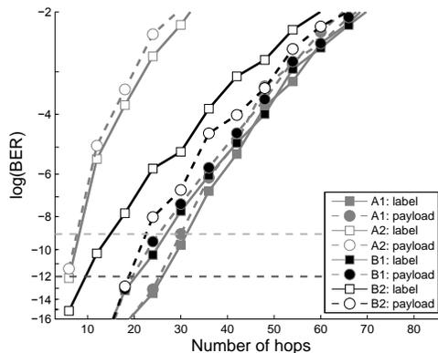
**Figure 5:** Scalability limits for the modified configurations after introduction of additional preamplifiers for label and payload.
