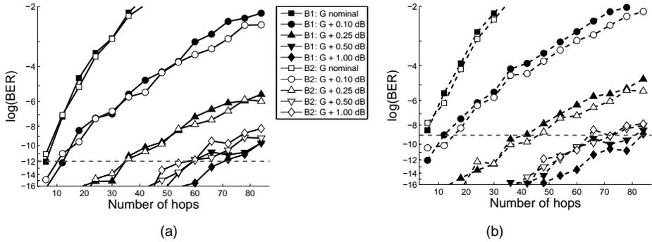
**Figure 6:** Scalability limits for (a) label and (b) payload for configurations B1 and B2 with 50/50 couplers. Different gain factors have been evaluated ranging from nominal G to G + 1 dB.
