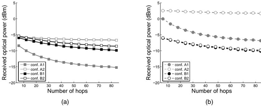
Figure 3: Received optical power for (a) label and (b) payload as a function of the number of hops.
