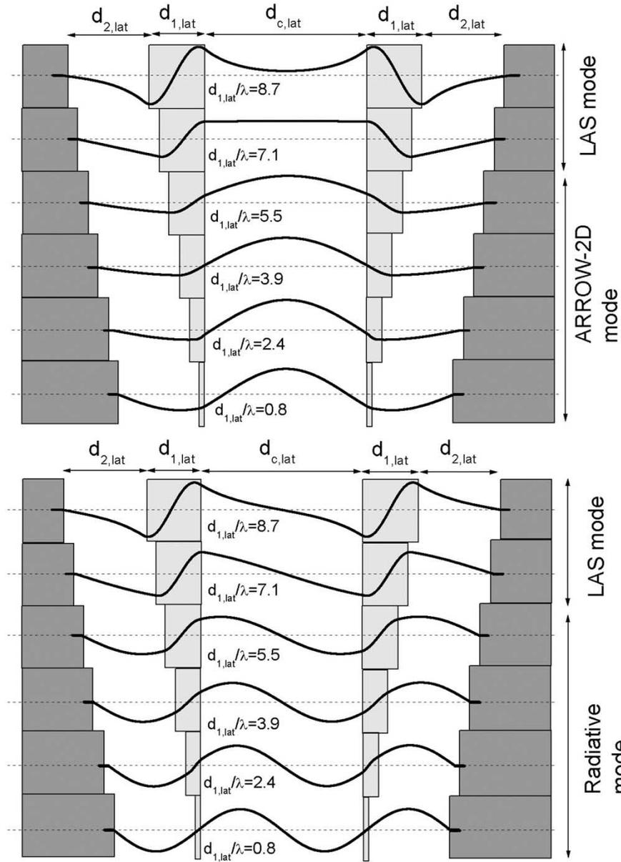
Fig. 4. Transformation of field profile of the  $\text{TE}_{\text{sym},1}$  and  $\text{TE}_{\text{as},1}$  as the  $d_{1,\text{lat}}/\lambda$  approaches the cutoff condition: symmetrical modes are transferred to the ARROW-2D modes, while asymmetrical modes are radiative modes below cutoff.
