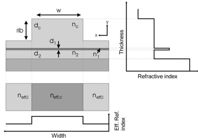
Fig. 1. Configuration and refractive-index profile of a rib-ARROW structure.
