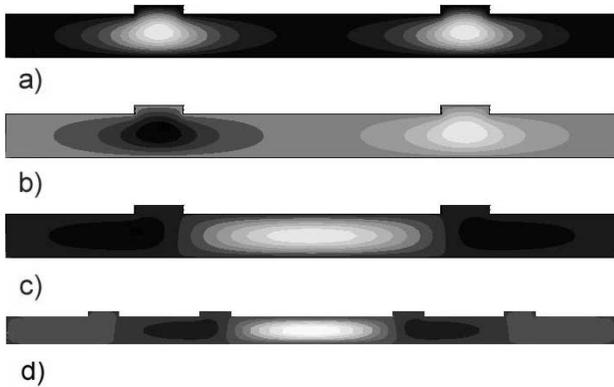
Fig. 5. Cross-sectional electric-field profiles of an ARROW 2-D structure with LAS structure at its first antiresonant condition ( $d_{c,lat}/\lambda = 4.67$ ): (a)  $TE_{sym,0}$ , (b)  $TE_{as,0}$ , (c) ARROW-2D mode, and (d) ARROW-2D mode in an ARROW-2D structure with double LAS.
