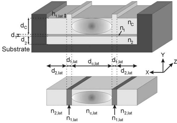
Fig. 2. ARROW-2D waveguide with single LAS and effective-refractive-index-equivalent slab structure. The thicknesses of the layers are  $d_c = 3 \mu\text{m}$ ,  $d_1 = 0.35 \mu\text{m}$ , and  $d_2 = 1.5 \mu\text{m}$ , while the refractive indexes are  $n_c = 1.462 \mu\text{m}$ ,  $n_1 = 2.00 \mu\text{m}$ , and  $n_2 = 1.46 \mu\text{m}$ .
