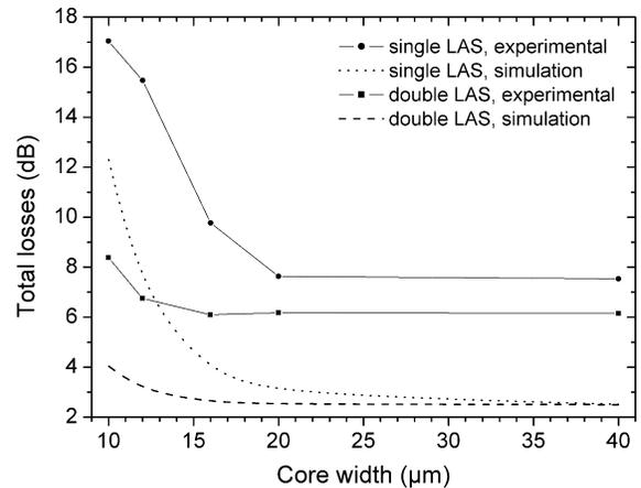
Fig. 6. Experimental and simulated losses as a function of the waveguide width ( $d_{c,lat}$ ) for ARROW-2D structures with single and double LAS.
