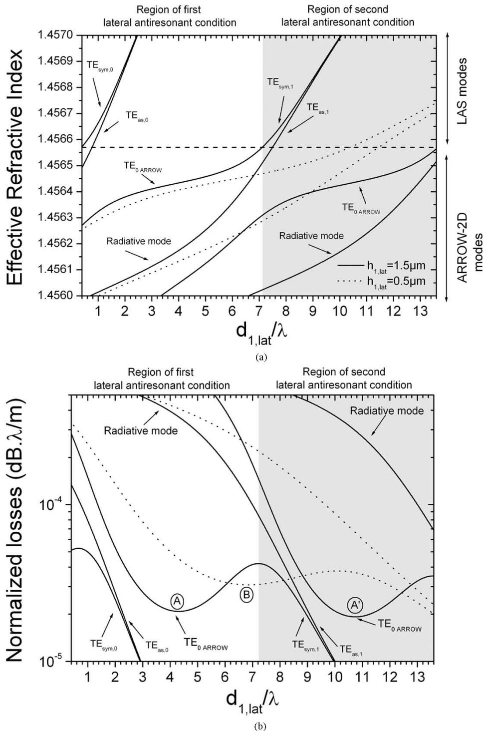
Fig. 3. (a) Effective refractive index and (b) normalized losses of a 16- $\mu\text{m}$ -wide, 3- $\mu\text{m}$ -thick ARROW-2D structure working at 633 nm for two different LAS heights ( $h_{1,\text{lat}}$ ). Transition between the symmetrical mode of the LAS ( $\text{TE}_{\text{sym},1}$ ) and the ARROW-2D mode ( $\text{TE}_{0,\text{ARROW}}$ ) is observed at lateral antiresonant condition.
