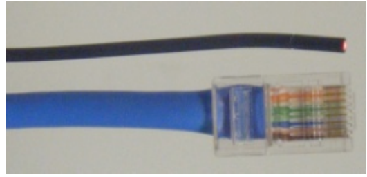
Fig. 4. POF and RJ45 cooper cable.
