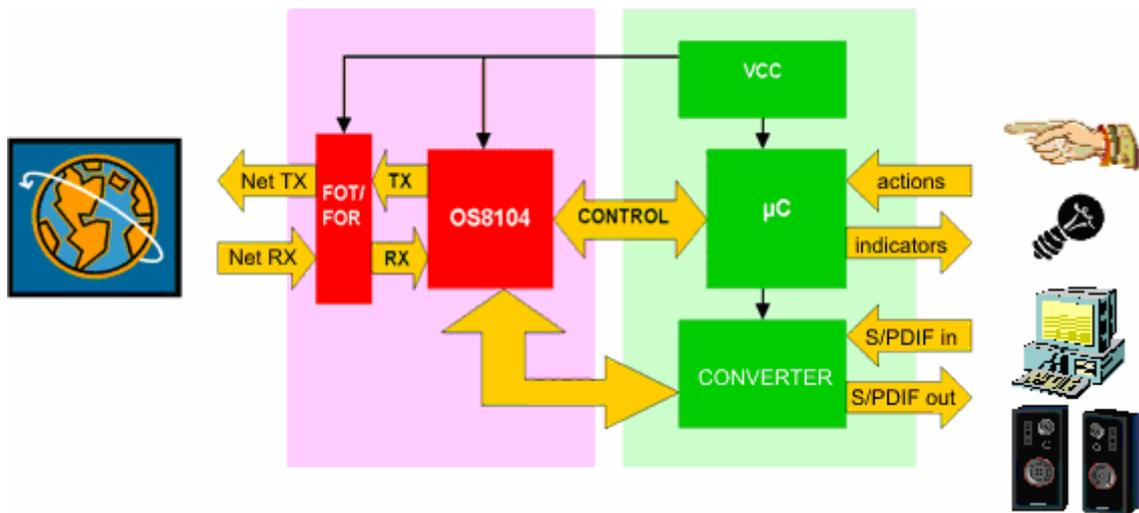
Fig. 1 a) Block diagram of the basic node with the Physical layer board (PLB) on the left and the application firmware board (AFB) on the right, showing their external connections and functions.
