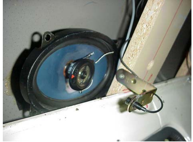
Figure 6. (a) Physical disposal of electro-acoustic elements. (b) Error microphone and secondary source.
