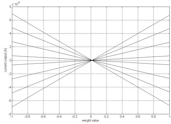
Fig. 4. Mixed-mode four-quadrant multiplier output
