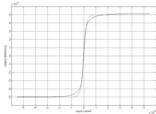
Fig. 6. Non-linear output function: Ideal (dotted line) and real (continuous line)
