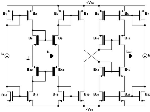
Fig. 3. Class AB activation function
