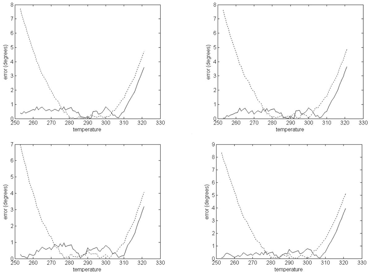
Fig. 11. NTC output error compared to neural network output error for four different NTC sensors
