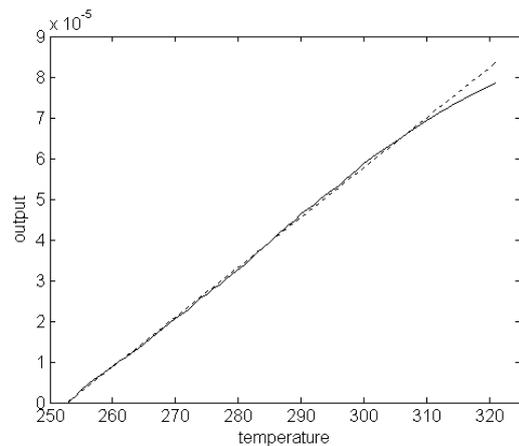
Fig. 10. Corrected output voltage versus ideal linear output
