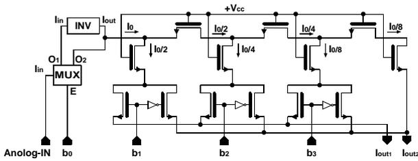
Fig. 2. Only three-bit four-quadrant mixed analog-digital multiplier (ADM)
