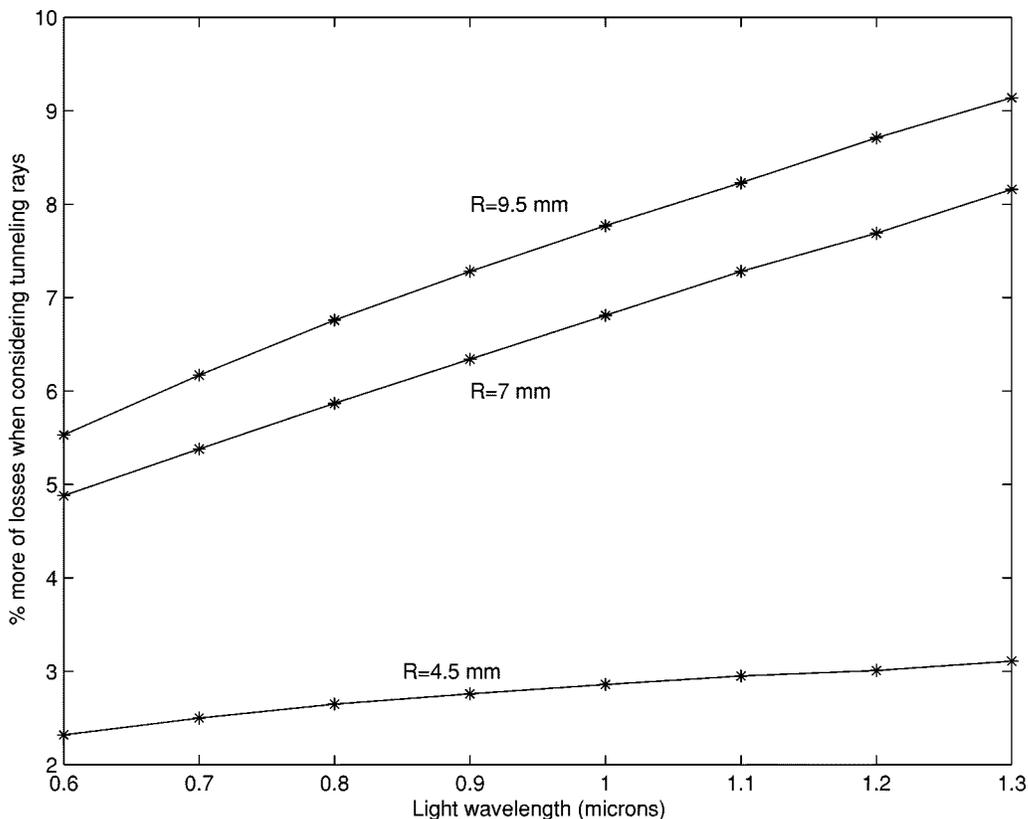
Fig. 3. Percentage of additional losses that would be obtained with the “Lucina” fiber ( $a = 65 \mu\text{m}$ ) when considering tunneling rays for 1-1/4 turns and different bend radii as a function of the light wavelength.
