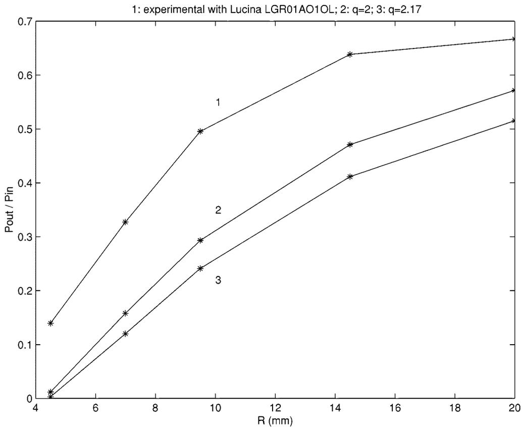
Fig. 8. Comparison between the experimental and the computational results obtained for the "Lucina" fiber as a function of the bend radius for 1-1/4 turns. 1: experimental; 2: theoretical for  $q = 2$ ; 3: theoretical for  $q = 2.17$ .
