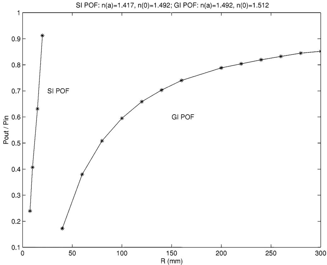
Fig. 6. SI POF: experimental results obtained for a typical step-index PMMA POF for one turn, as a function of the bend radius, shown for the sake of comparison with graded-index POF. GI POF: output power relative to the input power obtained for a 1-mm-diameter GI PMMA POF as a function of the bend radius for 1-1/4 turns.
