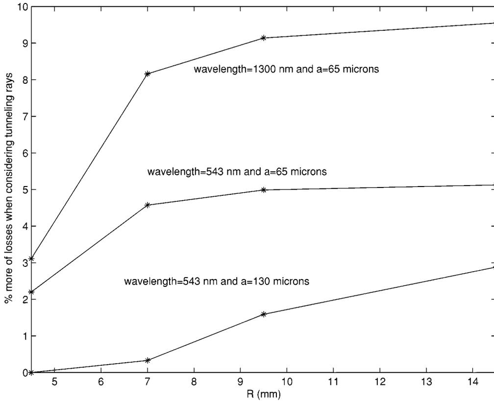
Fig. 4. Combined influence of the light wavelength and the fiber core radius  $a$  on the “Lucina” fiber as a function of the bend radius for 1-1/4 turns.
