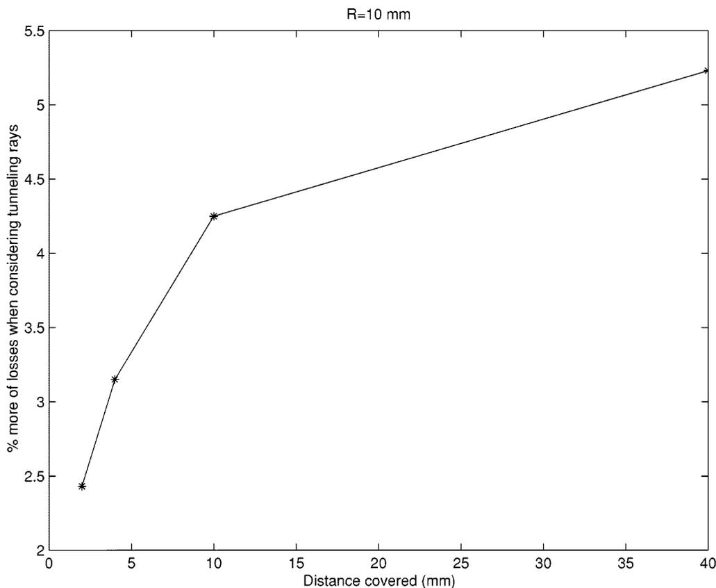
Fig. 5. Percentage of additional losses that would be obtained with the “Lucina” fiber (Lucina LGR01AO1OL) when considering tunneling rays as a function of the distance covered around a cylinder of fixed bend radius (10 mm).
