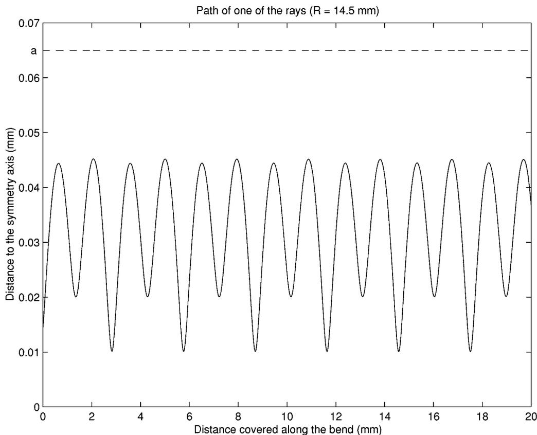
Fig. 1. The path of one of the numerous rays considered to study the radiation losses for a bend radius of 14.5 mm, in the case of profile exponent equal to two, core radius of 0.065 mm, and core and cladding refractive indexes equal to 1.353 and 1.340, respectively. For this ray,  $\beta = 1.3482$  and  $l = 0.1179$ .
