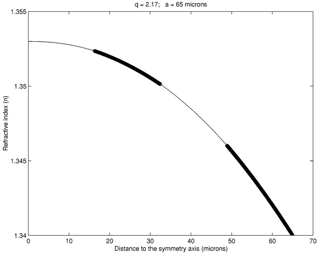
Fig. 2. Four parabolas of the form “ $a + cu^2$ ” can fit the core refractive index very approximately when the profile exponent  $q$  is different from two ( $q = 2.17$  in the figure). The exact refractive index has been plotted with a thin line and the second and fourth parabolas has been plotted with thick lines.
