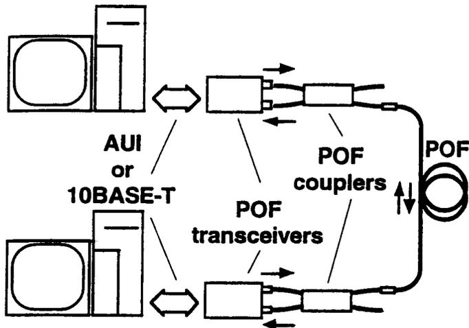
Figure 1.- Scheme of the bi-directional one-port POF link configuration
