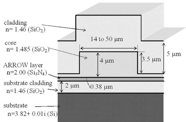
Fig. 2. Structure of the ARROW waveguides fabricated.
