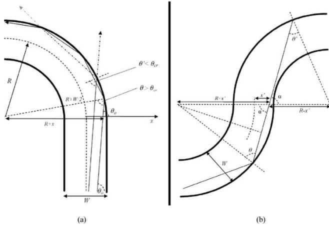
Fig. 3. (a) Ray tracing in the transition between a straight and a curved waveguide and (b) in the transition between two waveguides of opposite curvatures.
