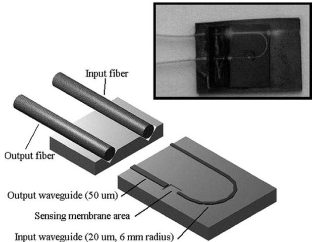
Fig. 1. Optochemical sensor employing bent ARROW waveguides (light outflow in the input waveguide of the photograph is not due to the transition between curvatures but to the fact that light is injected using a multimode waveguide to increase packaging tolerances).
