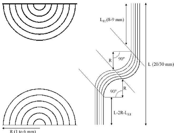
Fig. 4. Details from the masks employed in the fabrication of “C” and “S” waveguides. Total length of “S” chips is 20 mm for radii ranging from 1 to 3 mm, and 30 mm for larger radii.
