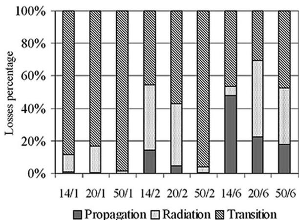
Fig. 5. Distribution of losses in the curved rib ARROW waveguides fabricated among the possible attenuation causes. W/R indicates a waveguide of rib width  $W$  and radius  $R$ .
