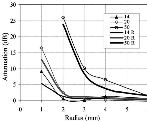
Fig. 6. Predicted (labeled with “R”) and measured total transition losses for different “S” waveguides at  $\lambda = 678$  nm.
