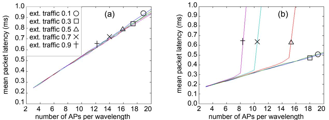
Figure 4. Mean packet latency versus number of nodes per internal wavelength for different external-to-internal traffic ratios for the internal wavelengths (a) and for the external wavelength (b).
