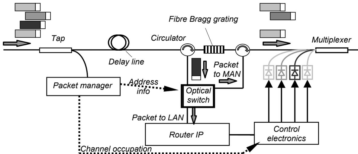
Figure 2. Access Point proposed design: every packet crossing the node suffers a delay introduced in order to avoid collisions with those packets added by the node. Additionally, packets belonging to the node's own wavelength cross the optical switch and are redirected either to the router (i.e. dropped) or again to the MAN ring.
