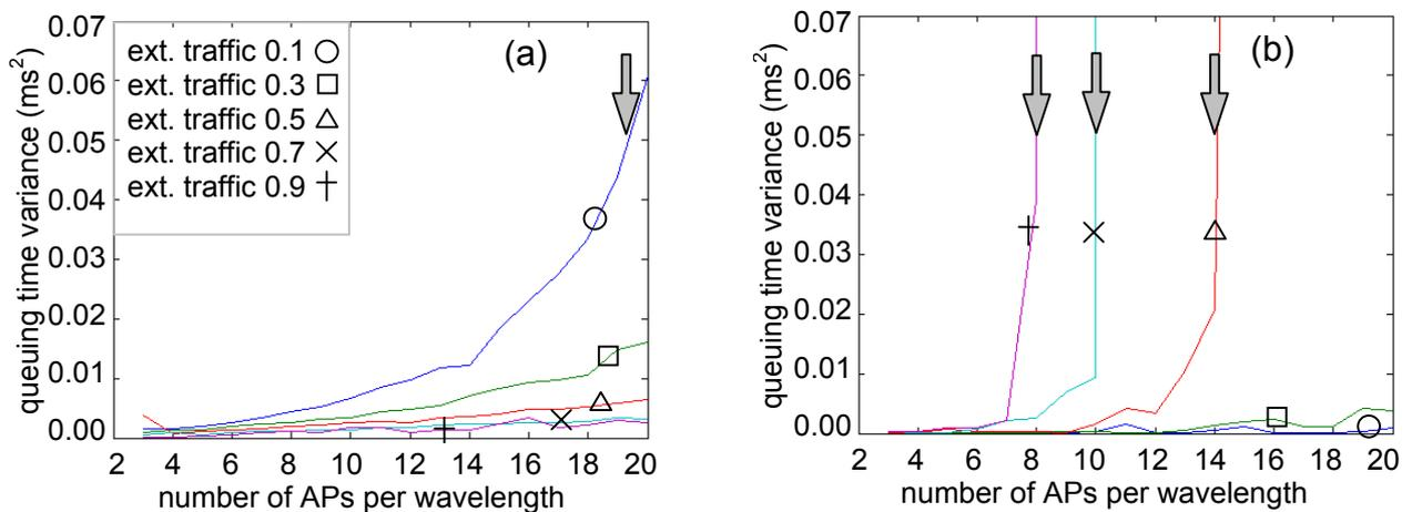
Figure 3. Queuing time variance versus number of nodes per internal wavelength, for the internal wavelengths (a) and for the external wavelength (b).
